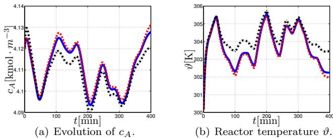
Fig. 3. Simulation results for the CSTR: nonlinear model (24) (red line), PWA approximation (26) (red dashed line), linear approximation (black dotted line).
