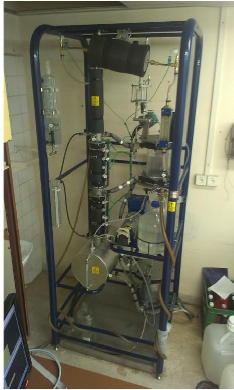
Figure 2.1: Laboratory Distillation Column
