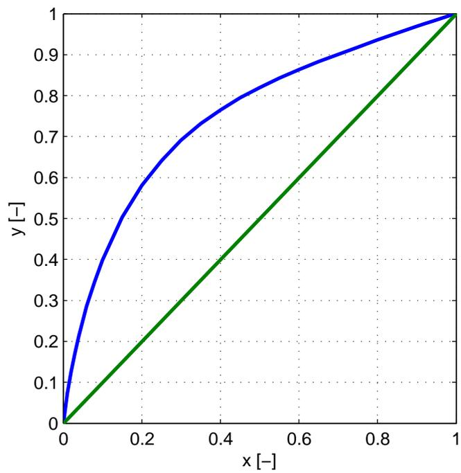
Figure 1.1: X-Y Diagram for mixture Methanol-Water
