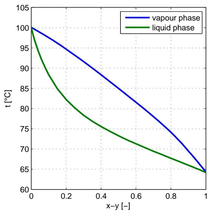
Figure 1.2: t-xy Diagram for mixture Methanol-Water
