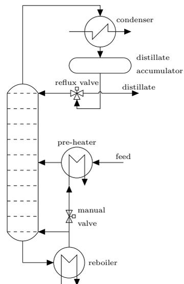
Figure 2.2: Scheme of Distillation Column
