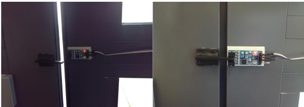
Figure 3.4 – Door opening sensor mechanism
