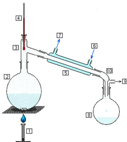
Picture 1 Simple distillation apparatus [17]
