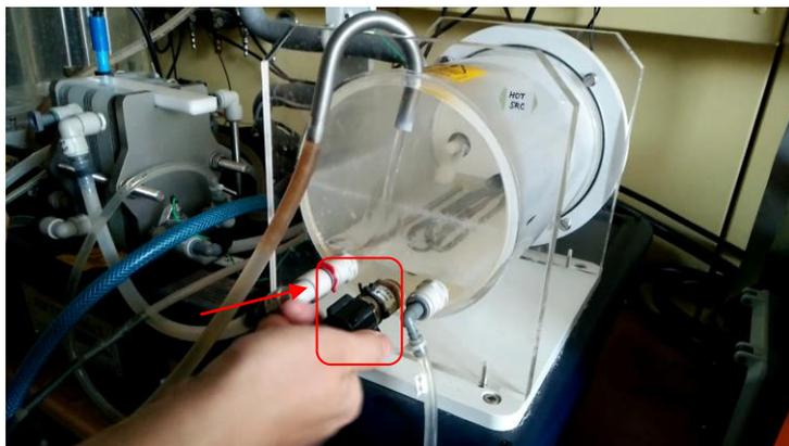
Picture 38 Closing the draining valve
