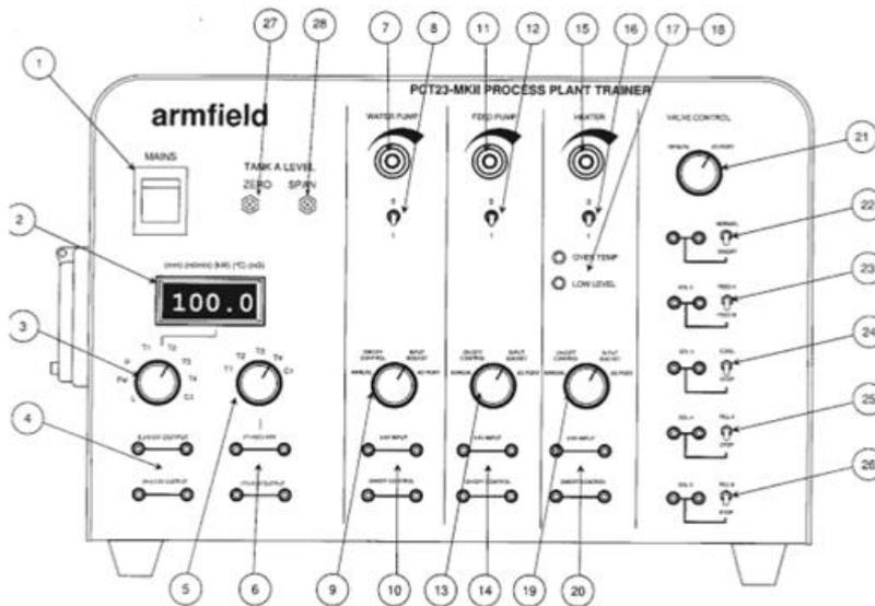
Picture 33 The front of the control console [3]
