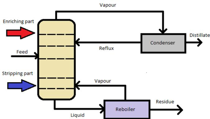
Picture 2 Schematic of a typical distillation unit [5]
