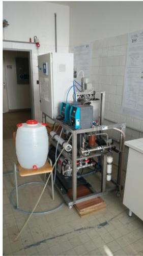
Picture 14 Batch membrane processing unit
