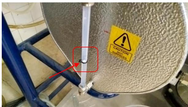
Picture 8 Liquid level in the reboiler
