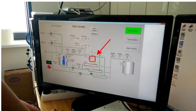
Picture 25 Turning on valve V1
