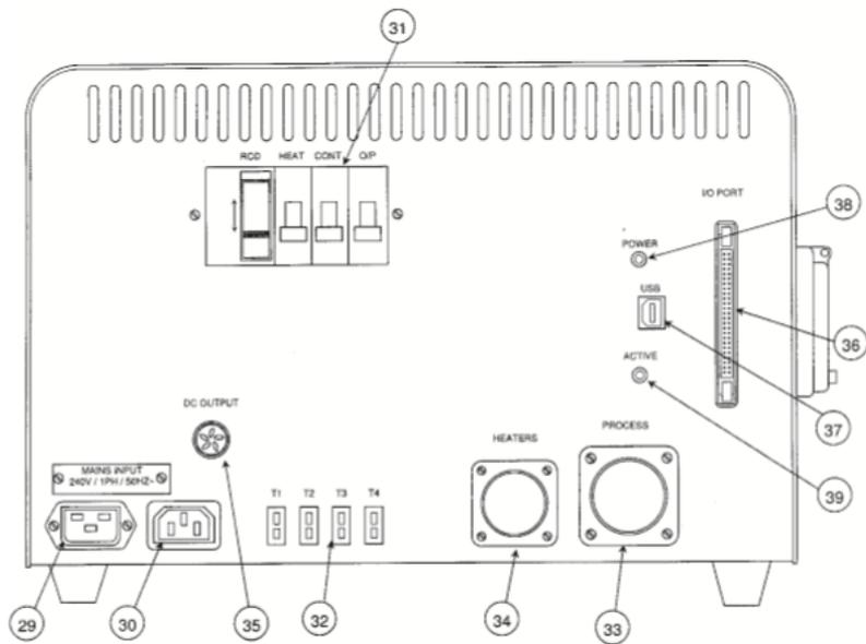
Picture 34 The rear of the control console [3]
