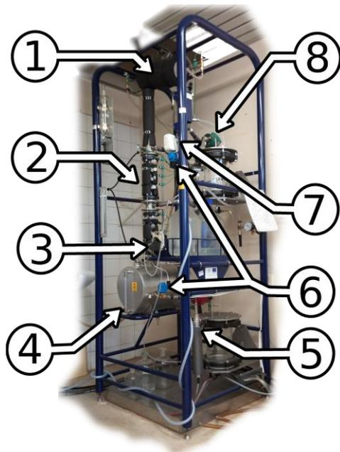
Picture 3 The UOP3CC distillation column [2]
