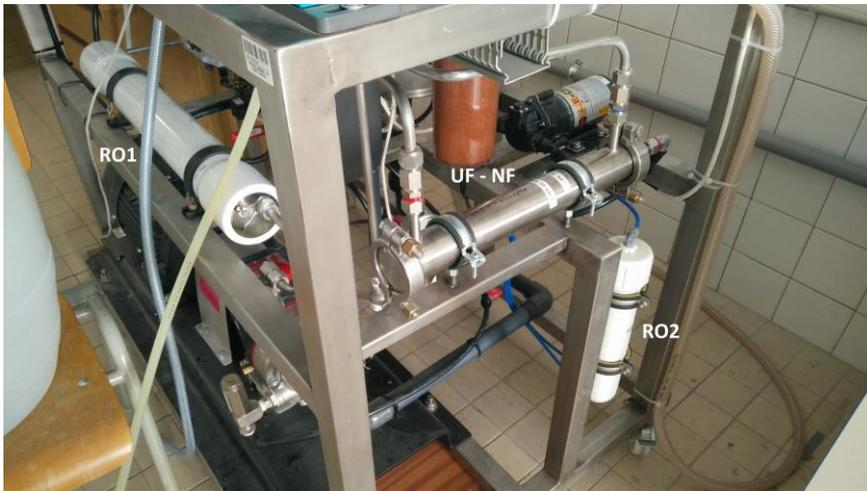
Picture 16 The filters of the unit
