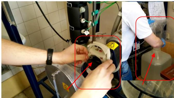
Picture 11 Feed tank and peristaltic pump
