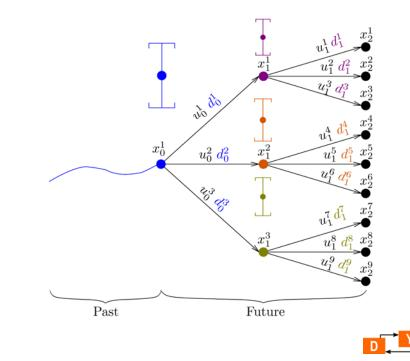
Comparison between different multi-stage NMPC using sigma point principles
