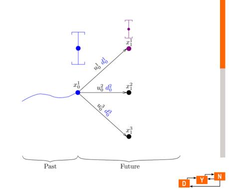
Proposed dual multi-stage NMPC using sigma points
