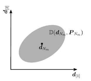
The new confidence region is used to reduce the uncertainty in the parameters and update the scenario tree of the multi-stage NMPC
