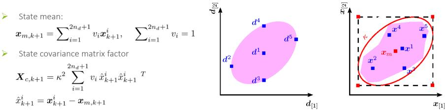
> The state covariance matrix can be scaled using the scaling factor  $\kappa$  such that the state ellipsoid encloses the reachable set of the model which is a tuning parameter<sup>[5]</sup>
