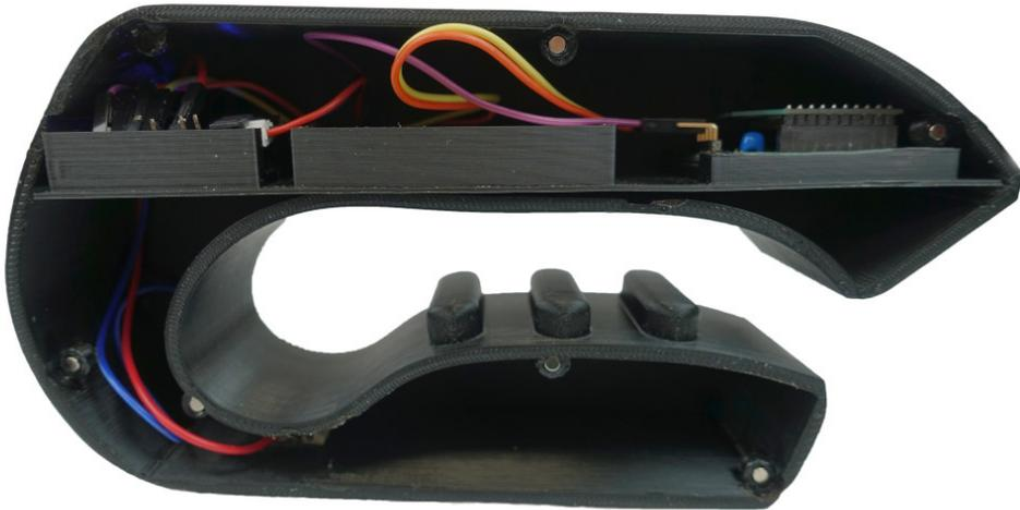
**Figure 4.2:** 3D printed controller cross section
