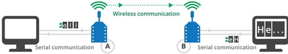
**Figure 4.11:** Types of data transmission in an XBee communication process[3]
