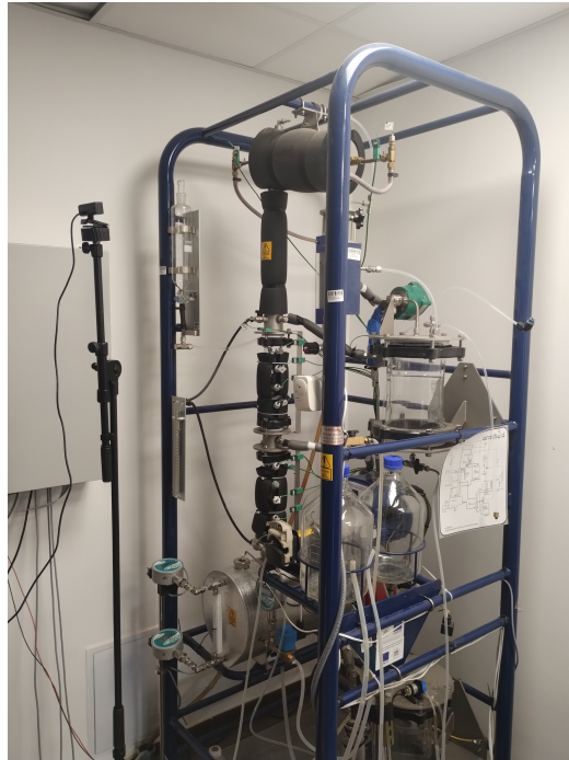
Figure 4.4: Distillation column with camera in school laboratory
