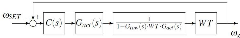
Figure 4.4 Modified control loop
