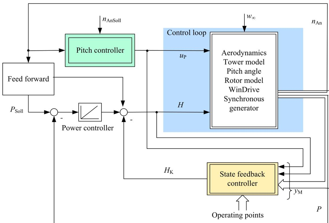
Figure 3.6 Control structure with detailed guide vane control
