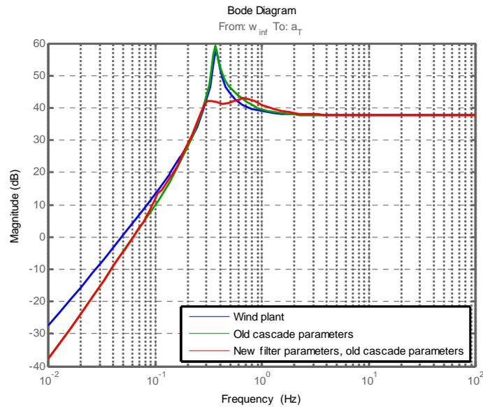
Figure 6.9 Frequency responses from the wind speed to the tower acceleration
