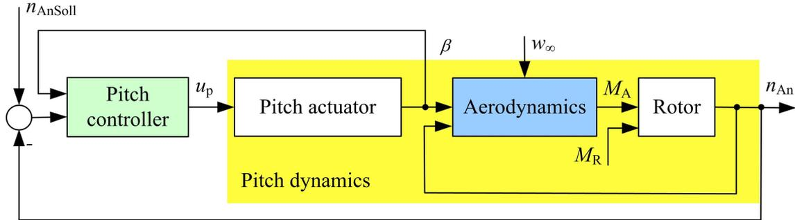
Figure 3.2 Pitch control loop
