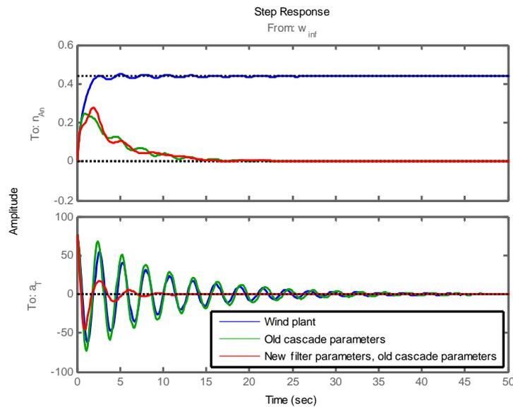
Figure 6.8 Step responses from the wind speed to the rotor speed and the tower acceleration
