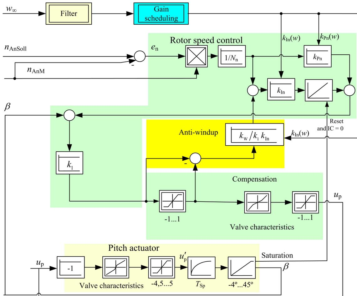
Figure 3.5 Realization of pitch control with gain scheduling and anti-windup
