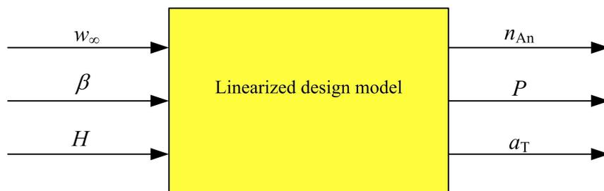
Figure 5.6 Simple structure of the linearized design model
