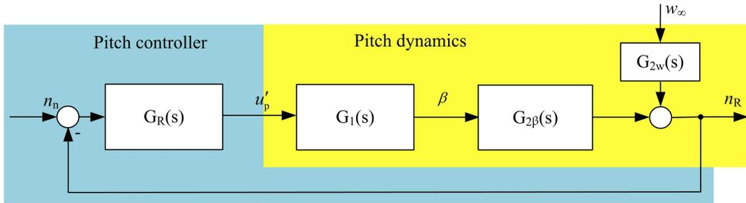
Figure 4.1 Principle scheme of the linearized wind turbine model [4]
