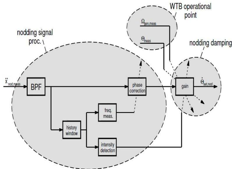
Figure 4.2 Control structure for improved damping of tower nodding [5]
