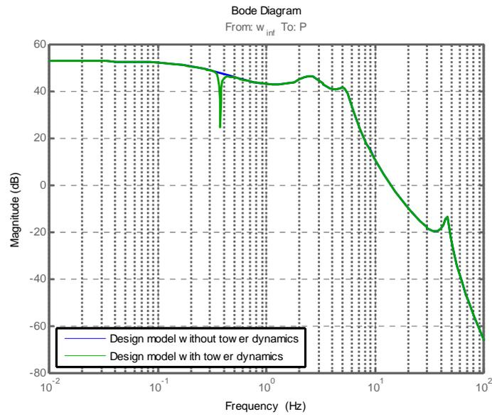
Figure 5.9 Frequency response of the wind speed to the power
