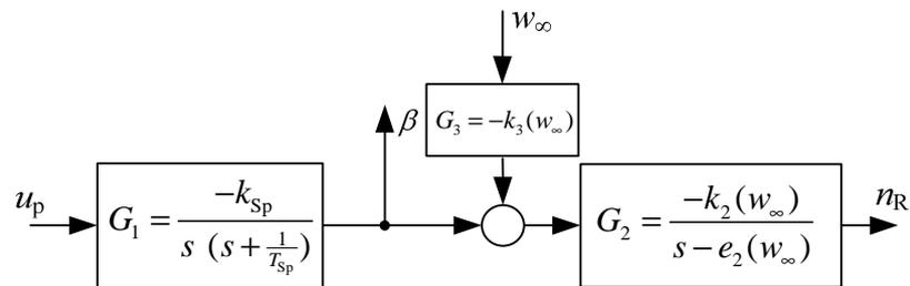
Figure 3.3 Linearized pitch plant
