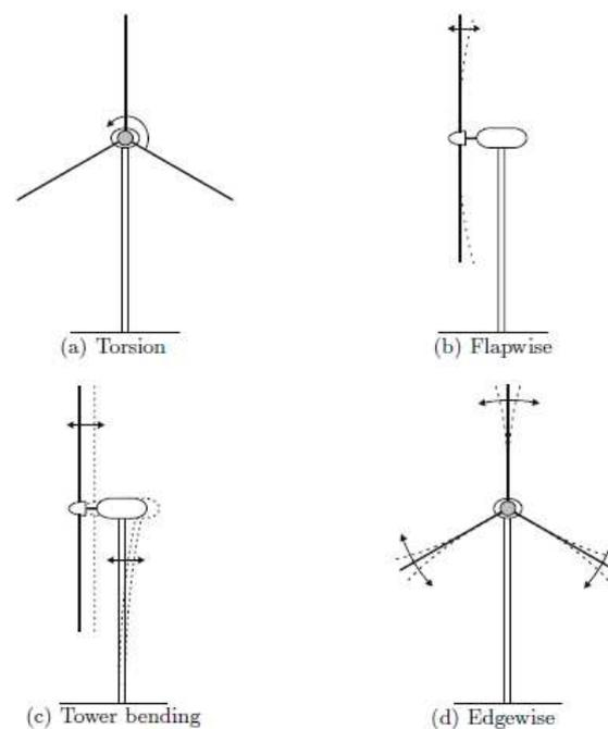
Figure 2.3 Oscillatory movements of the tower [1]
