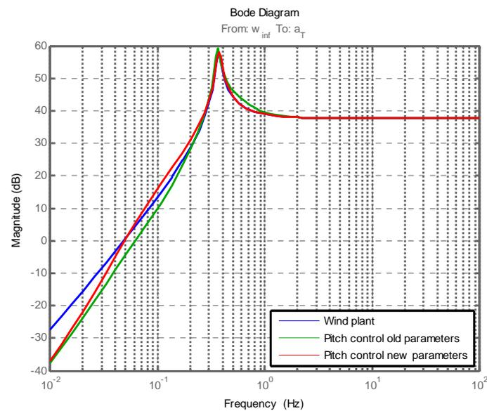
Figure 6.4 Frequency response from the wind speed to the tower acceleration
