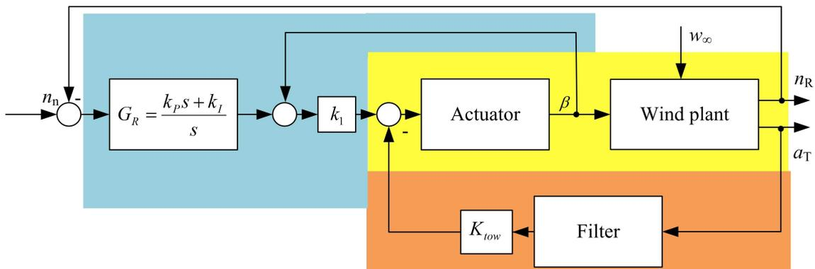
Figure 6.5 New pitch controller extended with acceleration feedback
