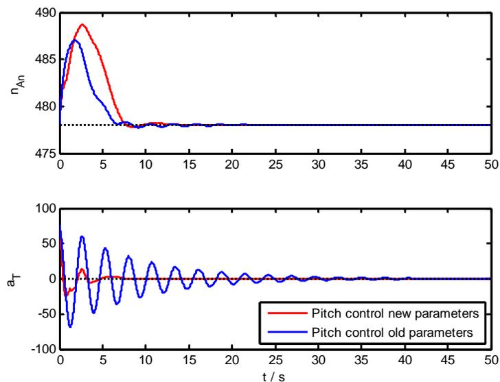
Figure 6.14 Step responses from the wind speed to the rotor speed and the tower acceleration, nonlinear system
