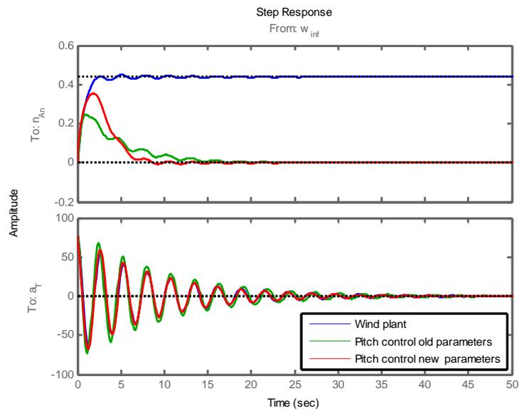
Figure 6.3 Step responses from the wind speed to the rotor speed and the tower acceleration
