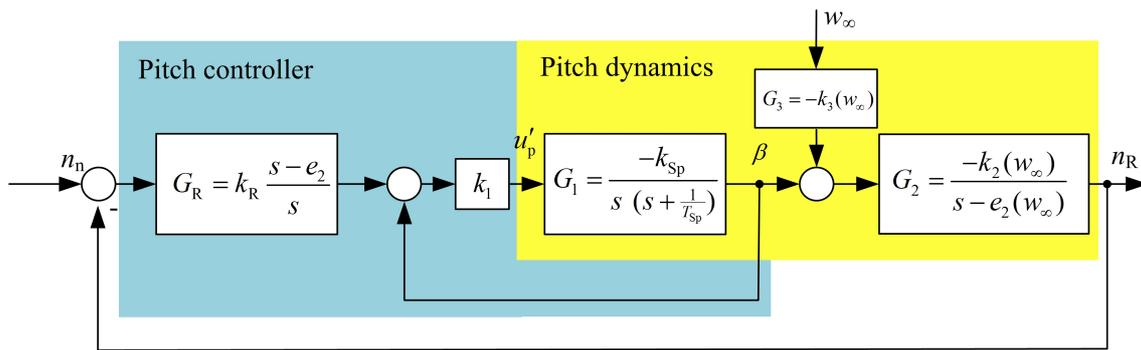
Figure 3.4 Pitch control using a P-PI cascade
