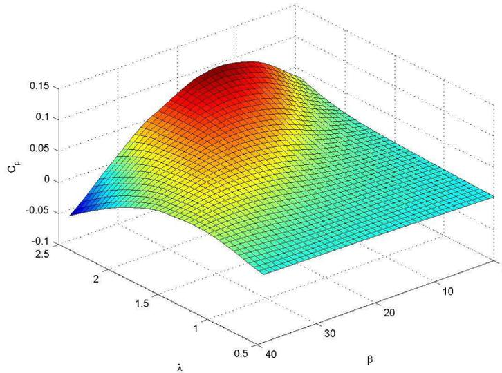
Figure 2.2 Variations of  $C_p$  for a wind turbine
