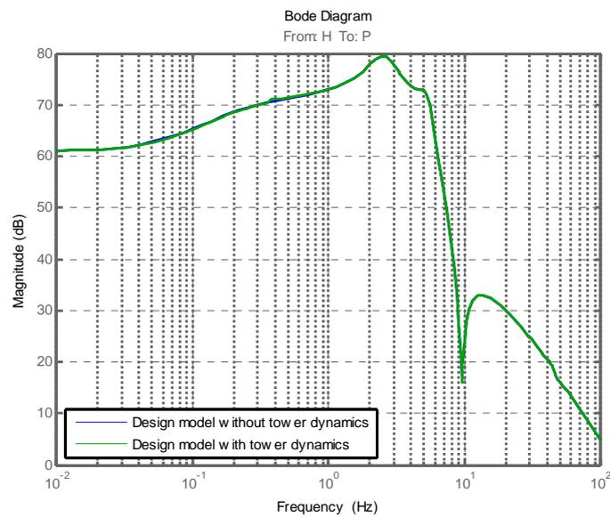
Figure 5.11 Frequency response of the guide vane position to the power
