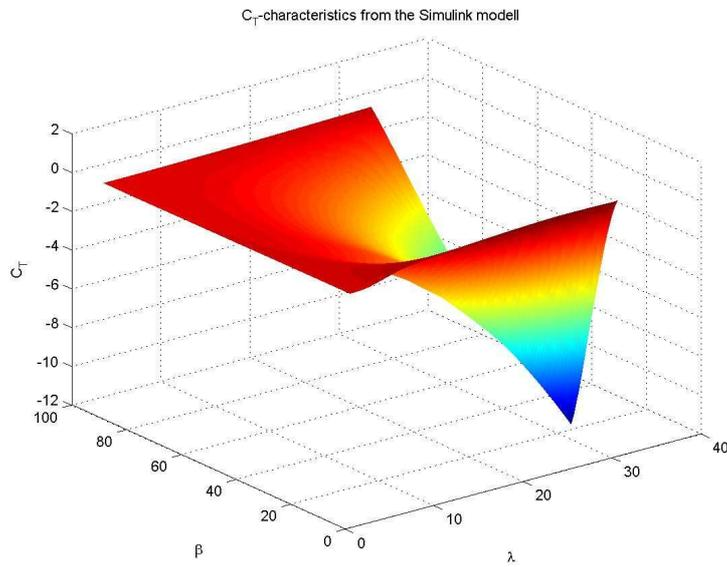
Figure 5.3 Generated C<sub>T</sub>-table
