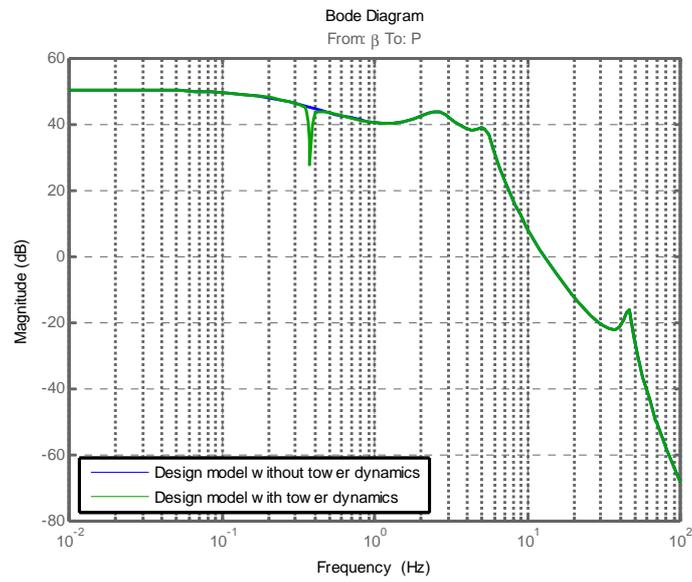
Figure 5.10 Frequency response of the pitch angle to the power
