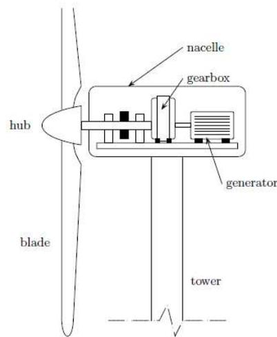
Figure 2.1 Example of a typical wind turbine [1]
