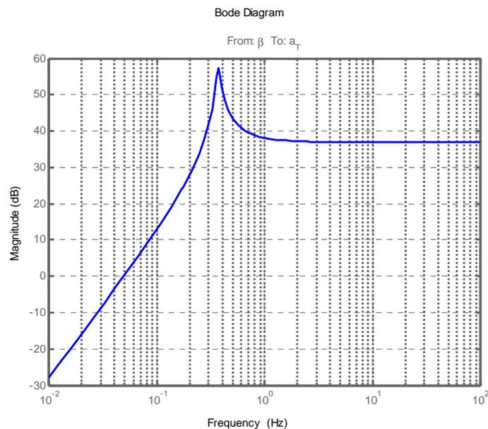
Figure 5.8 Frequency response of the pitch angle to the tower acceleration
