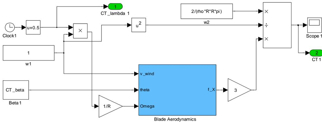
Figure 5.2 Simulink realization of the  $C_T$ -table generation
