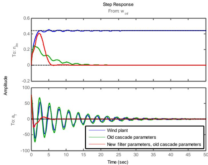
Figure 6.12 Step responses from the wind speed to the rotor speed and the tower acceleration
