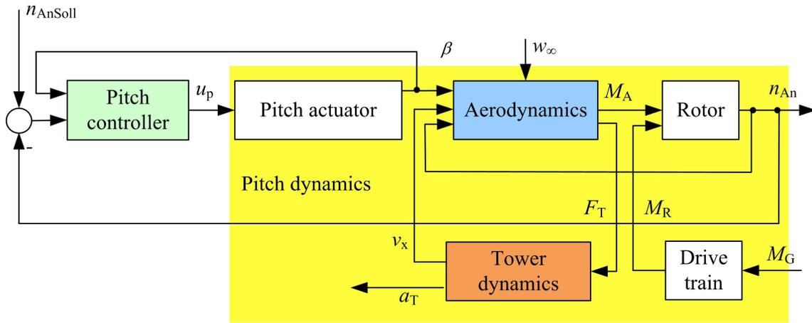
Figure 5.1 New design model extended with tower dynamics
