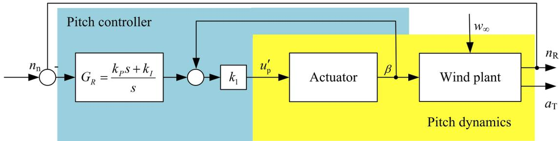
Figure 6.1 Pitch control using a P-PI cascade
