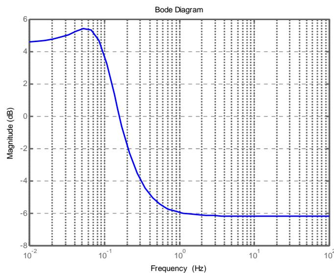
Figure 6.6 Second order Chebyshev filter with a 0.5 dB ripple
