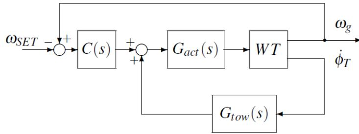
Figure 4.3 Inner loop for the cancelling of the tower fore-aft mode [6]
