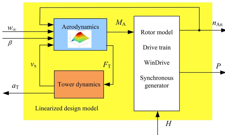
Figure 5.5 Linearized design model
