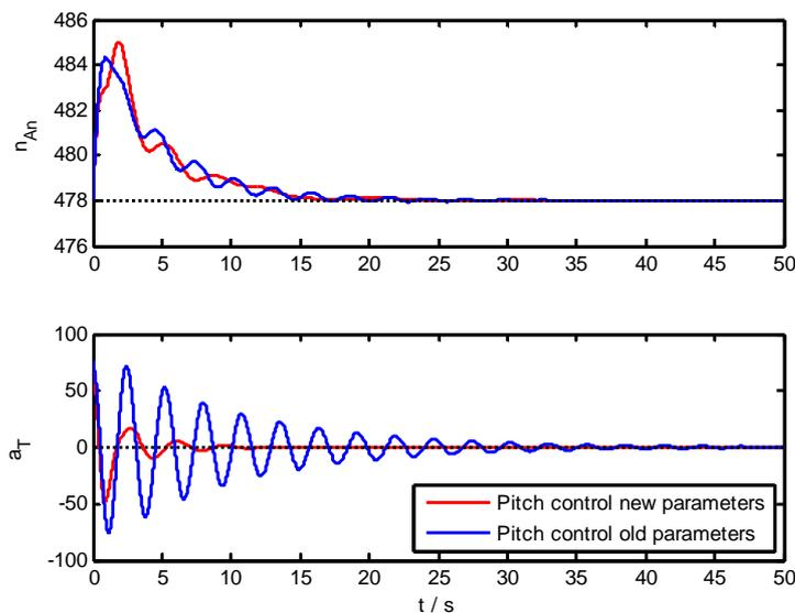
Figure 6.10 Step responses from the wind speed to the rotor speed and the tower acceleration, nonlinear system
