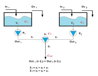
CIn2, C2, C3 and Cout) by considering dilution phenomena that can appear in the tank and at the interconnections. An important element is the behavior of the charges during powerful rain fall events. The final goal is to be able to minimize the charge overflow and not only the volume overflow.
