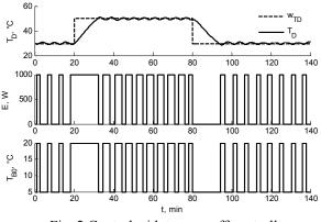
Fig. 2 Control with two on-off controllers
