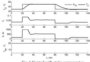
Fig. 6 Control with static compensator
