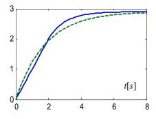
Fig. 5. Approximation of H(s) by a first-order plant
