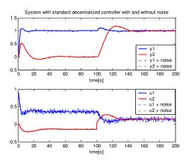
Fig. 3 System with standard decentralized controller with and without noise
