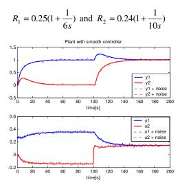
Fig.2 System with designed controller with and without noise
