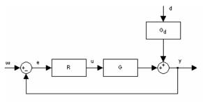
Fig. 1 Block diagram of feedback control system
