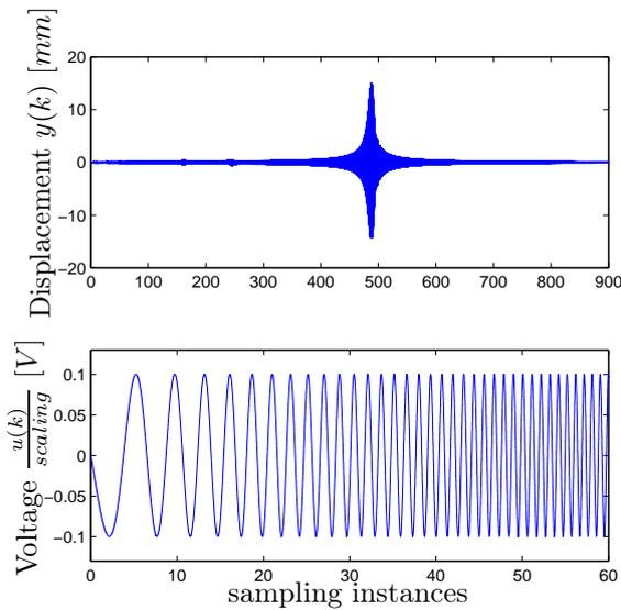
Fig. 2. Input/Output signals for system identification (*scaling* = 1000)
