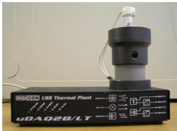
Fig. 1. Front view on a thermo-optical device uDAQ28/LT.
