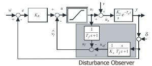
Fig. 1 DOB based PI<sub>1</sub> controller
