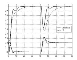
Fig.3 Transient responses of the PI controller tuned at the point (20) and the  $PI_1$  controller responses with tuning (22) for the actual plant parameters (21)
