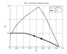
Fig. 2 Region of one-pulse of control of the PI<sub>1</sub> controller ( $T_{dr} = 0$ ) tuning outlined by the full curve and both axes: **•** - tuning (16) giving minimal IAE value for disturbance response, • - tuning (17) giving minimal ISE value for disturbance response; dotted – region of one pulse control for the predictive controller with the compensated time  $T_{dr} = 0.7T_d$
