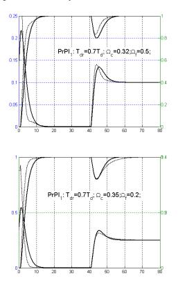
Fig. 5 Transient responses corresponding to the PI controller (7-9) (full) and to the predictive controller (Fig. 4) for two different tuning of the one-pulse control (dot)
