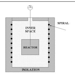
Fig. 1. Reactor furnace chart
