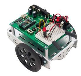
Fig. 1 Differentially steered mobile robot
