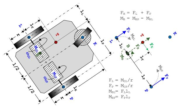
Fig. 3 Chassis scheme and forces
