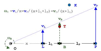
Fig. 4 Linear and angular speeds recalculations
