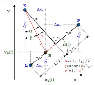
Fig. 5 Arbitrary chassis point recalculation
