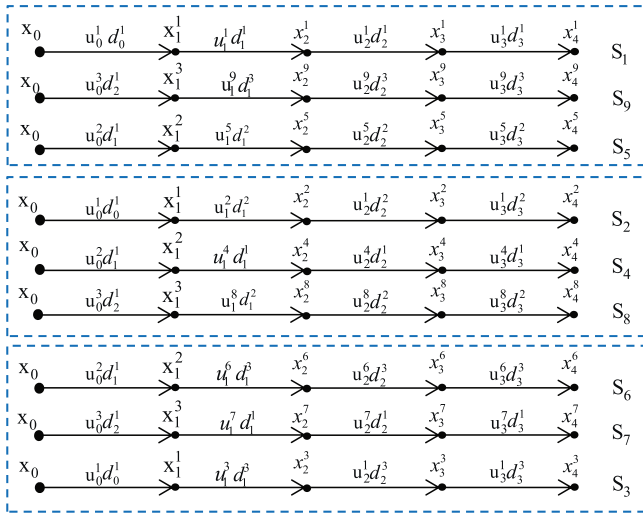
Fig. 3. Scenario tree representation of the uncertainty evolution using bundle decomposition for multi-stage NMPC. The scenarios in the same box represent the bundles.
