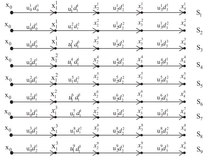
Fig. 2. Scenario decomposition representation of the uncertainty evolution for multi-stage NMPC.
