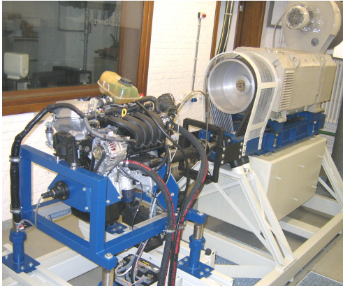
(a) Combustion engine connected to an electrical brake
