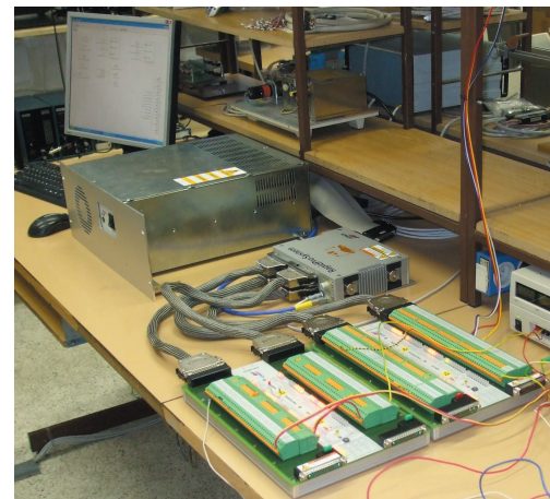
Fig. 1. Hardware assembly of the workbench
