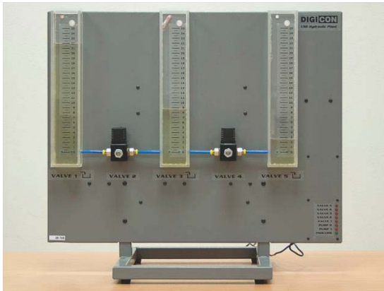
Fig. 6. Real three-level hydraulic plant.
